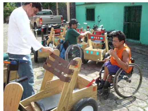
The new leather backs give more comfort and leg room to the PET.
